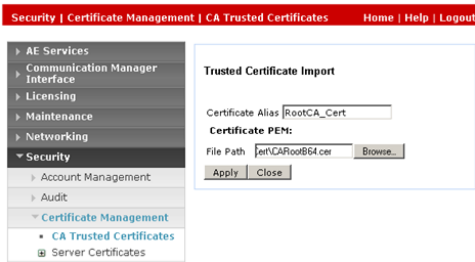
Figure 24: Example of importing a CA Trusted Certificate into AES
