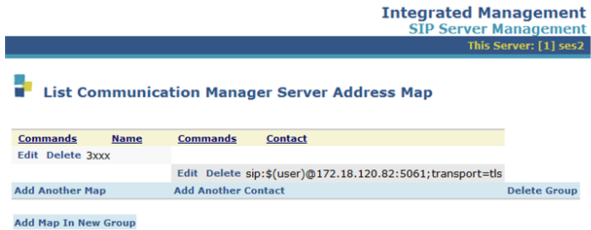
Figure 11: Example of routing entry or address map to Communication Manager
