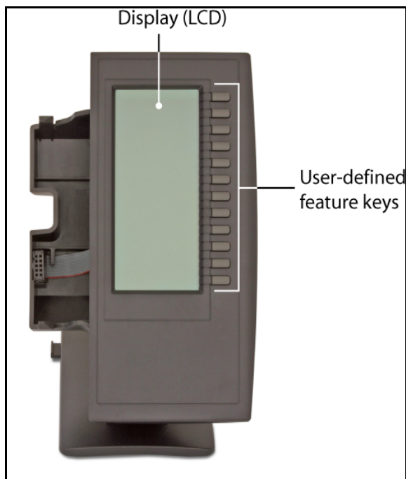
Figure 9: LCD Expansion Module (12-key self-labeling)
