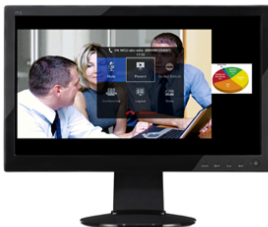
Figure 4-9 Showing the monitor in PoP view
