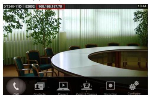
Figure 49: IP address displayed on the XT Series monitor
