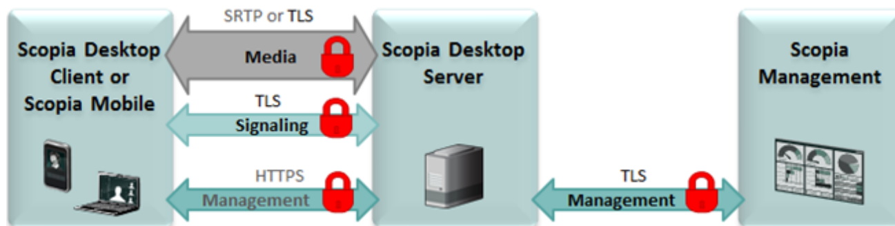
Figure 69: Encrypting communications using TLS
