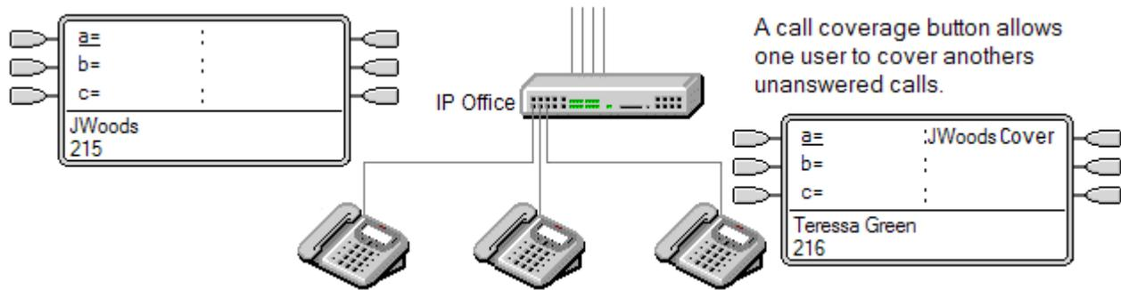
The user being covered does not necessarily have to be a key and lamp user or have any programmed appearance buttons. Their Individual Coverage Time setting (default 10 seconds) sets how long calls will alert at their extension before also alerting on call coverage buttons set to that user.
