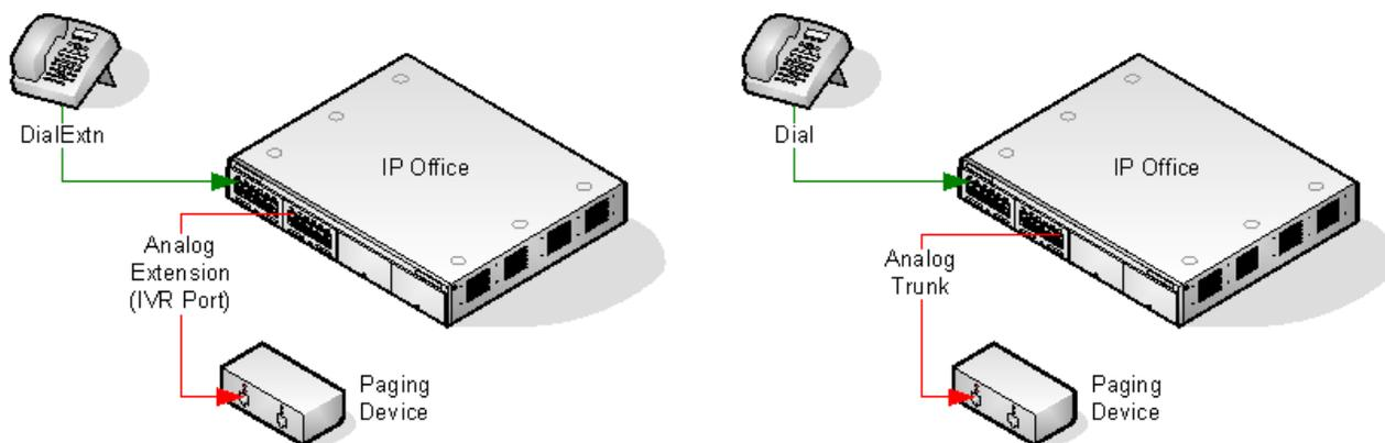
Uses a paging interface device such as a UPAM or amplifier with analog trunk/extension interface. The device can be connected to an analog trunk port or analog extension port.
