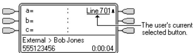
On phones with twin LED lamps, the current selected button is indicated by the red lamp being on
