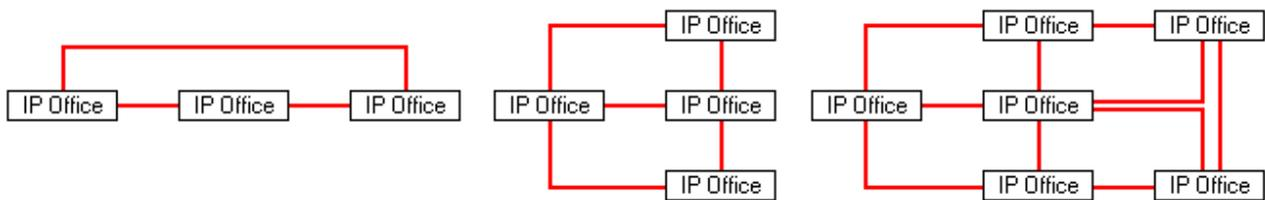
**Small Community Network Signalling** Small Community Network uses a signalling similar to RIP in order to update each other of their presence. This traffic can be seen in the System Monitor application as AVRIP packets. This traffic is sent to port 50795 on which each system listens.
