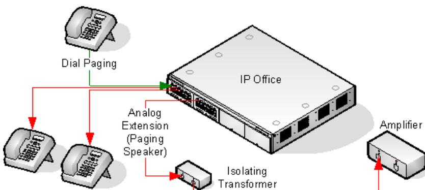
Uses an amplifier connected to an analog extension port via a 600ohm isolating transformer. Some amplifiers include an integral transformer. Avaya/Lucent branded amplifiers are designed for connection to special paging output ports not provided on systems. They are not suitable for supporting mixed paging.
