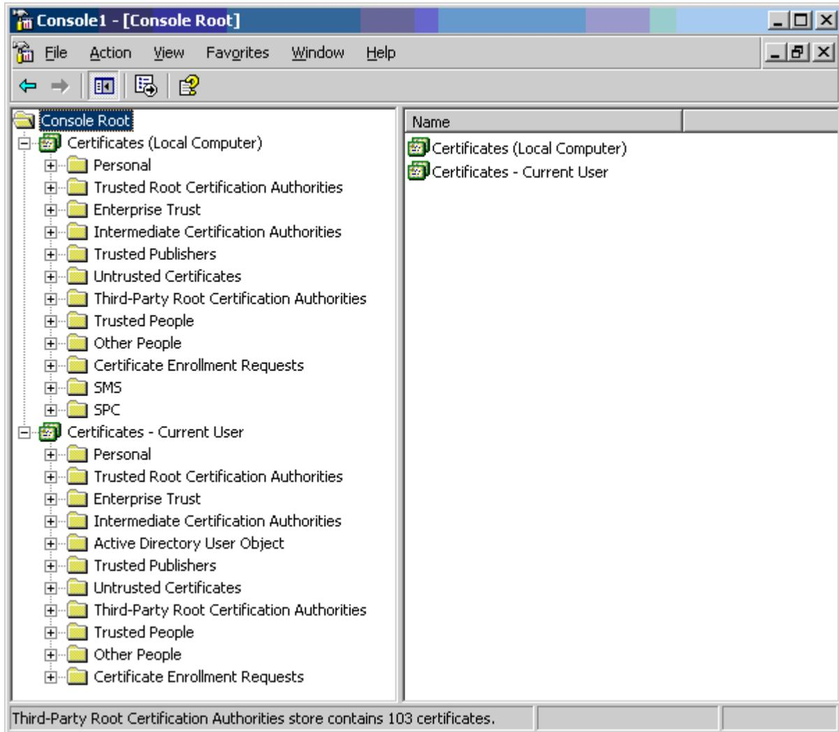
Each of the sub folders has differing usage. The Certificates - Current User area changes with the currently logged-in windows user. The Certificate (Local Computer) area does not change with the currently logged-in windows user.
