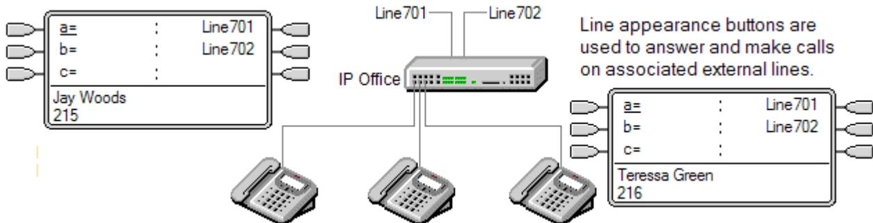
Incoming call routing is still used to determine the destination of all incoming calls. Line appearance buttons allow a call on a specific line to alert the button user as well as the intended call destination. When these are one and the same, the call will only alert on the line appearance but can still receive call coverage.
