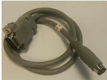
Figure 22: Camera Output, Cable Adapter to Kramer TP-573
