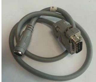
Figure 21: XT Camera Input, Cable Adapter to Kramer TP-574
