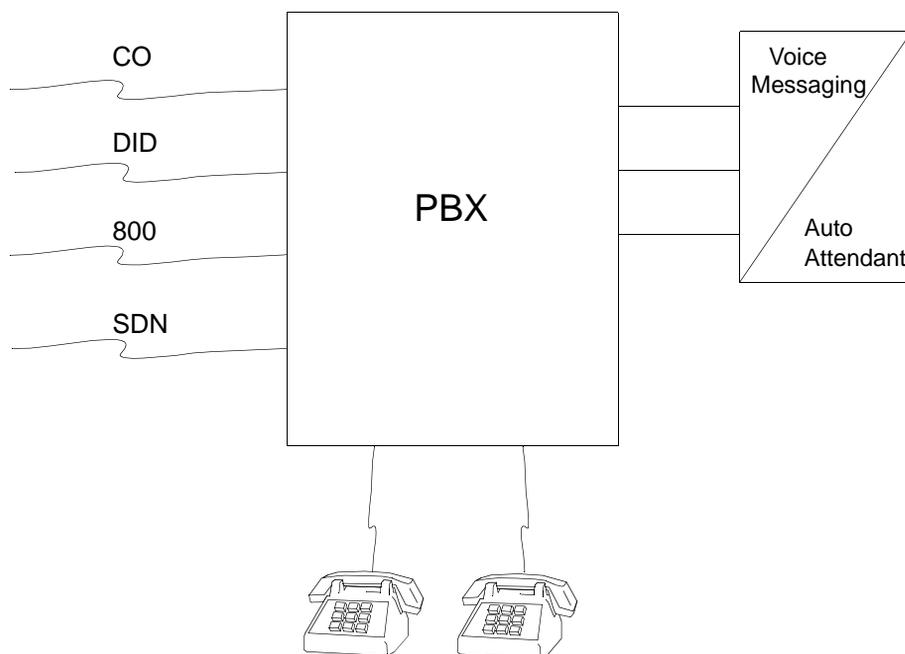
**Figure 6-1. Call Transfer Through the PBX**
