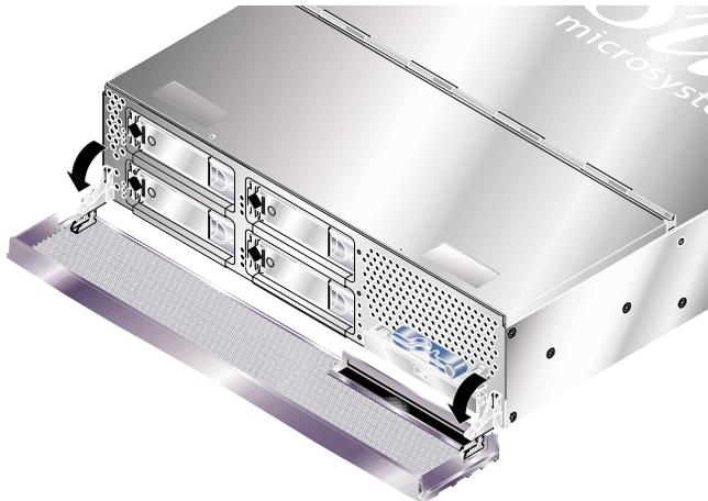
FIGURE 2-2 Opening The Bezel on a Sun Fire V210 Server
