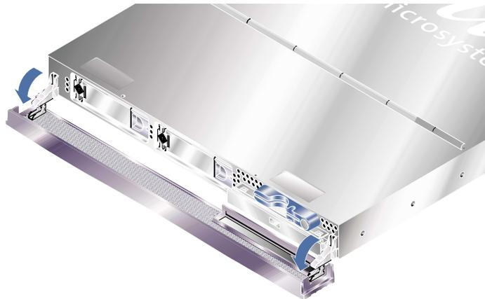
FIGURE 2-1 Opening The Bezel on a Sun Fire V210 Server
