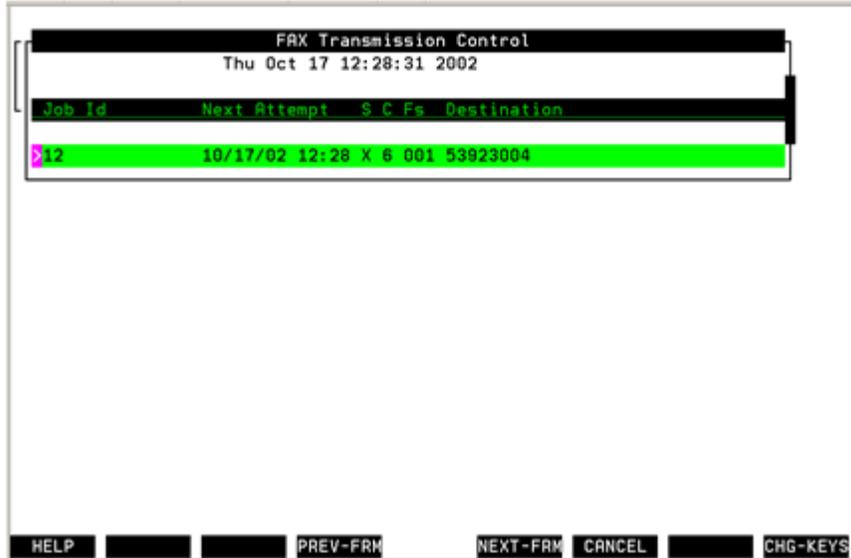
The **FAX Transmission Control** window lists the details (such as time, date, and size) for every fax job in queue. The fax jobs are listed in the order in which they appear in the fax transmission queue.
