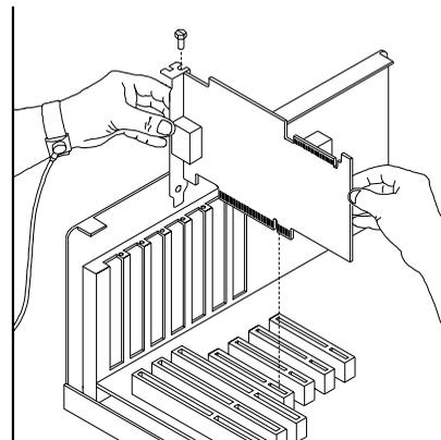
5. Install the retaining screw.
