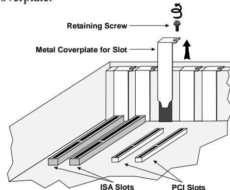
4. Insert the board's edge connector into the bus slot. Apply pressure only to the top edge of the board, and gently rock the board forward and backward to seat the edge connector into the slot.
