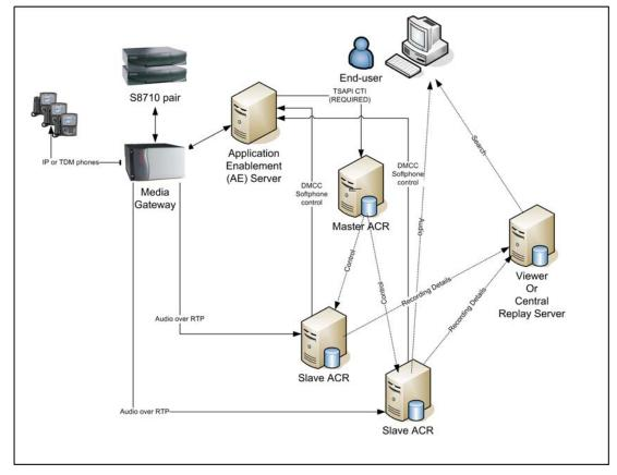
The Master recorder communicates with each Slave via a TCP/IP link. It instructs the slaves to tag the required data/voice streams with the details it learns from the CTI link. Preferably, one of the slave recorders is actually designated as a "Standby" recorder and can take over should the Master fail (though this requires additional backup channel licenses). All active recorders load balance at all times, regardless of which is in control.
